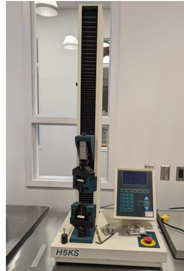
Hounsfield Materials Tester Model H5KS (Load capacity is 5kN with a speed range from 0.01 to 1000 mm/min)
