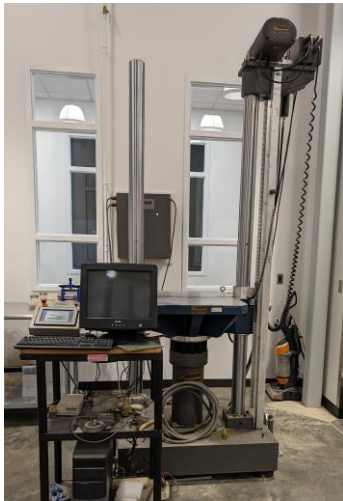
Lansmont Shock Tester Model 65/81 (500-lb capacity)
