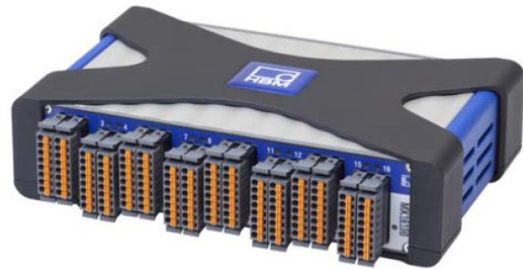
HBM QuantumX MX 1615B Strain Guage Bridge Amplifier (16 channels with data rate up to 600 20kS/s per channel, full-, half-, or quarter-bridge 120 or 350 Ohm)
