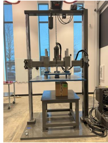
Lansmont 122-15 Compression Tester (48-in W x 48-in L x 78-in H maximum package dimensions, 1,500 lb – 15,000 lb force range)
