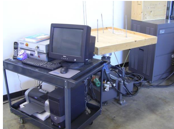
Lansmont Model 1000 Vibration Test System (75-lb capacity)
