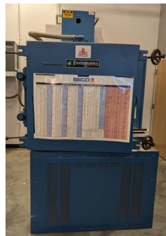
Envirotronics Altitude Chamber Model EA8-2-3-AC (-90F to +350F, Up to 100000 ft altitude, 24"x24"x24" chamber size)
